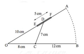
The point D slides along a fixed bar EF. When the window is closed, D is at F. When the window is fully open, D is at E.
